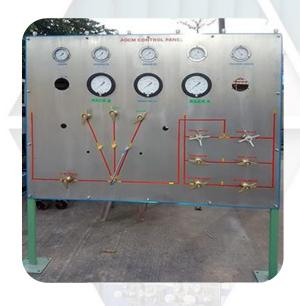
Hydrostatic Test Station is a way in which pressure vessels such as Gas Cylinders, Pipeline, Gas Handling Systems can be tested for strength and leaks. Vessel is filled with a fluid, mostly water and pressurised using a hydraulic pump to the specified test pressure.
